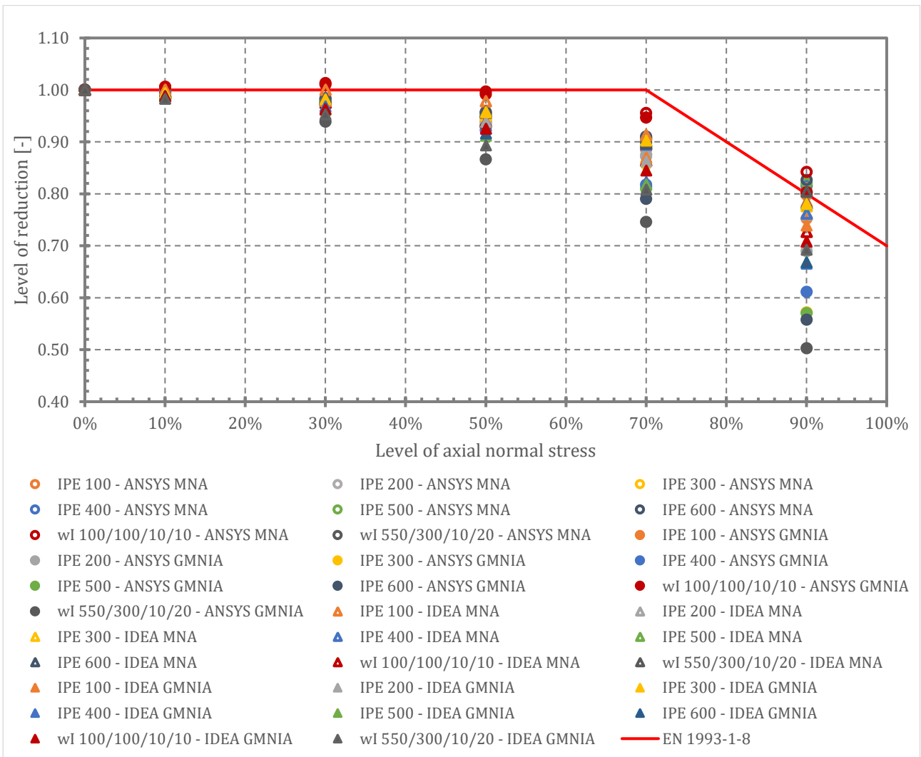
Fig. 159 Influence of normal force – relative influence of axial force on load-carrying capacity
