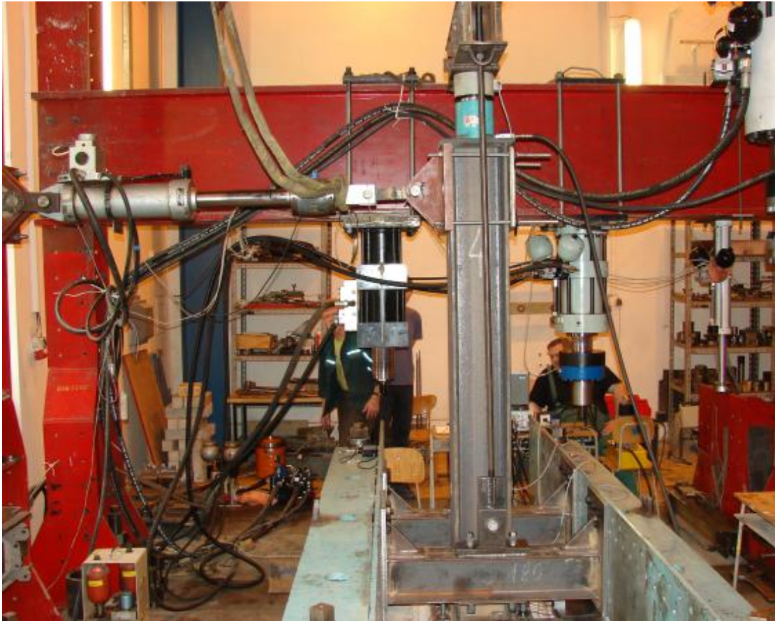
Figure 3: The test set-up of joint 2 — axial force and in-plane bending
