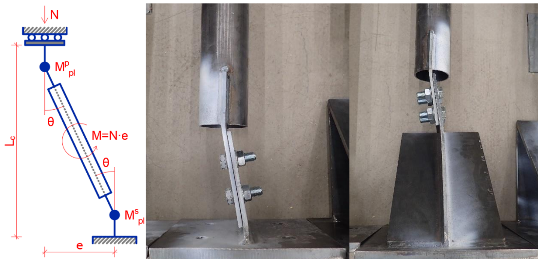
Figure 4: Failure mode of eccentric gusset plate connection (Vesecký, 2019)
