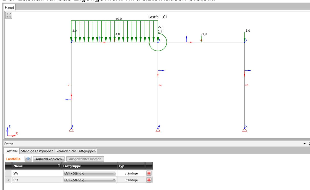
The screenshot displays the main window of the IDEA Frame software. The top part shows a 3D structural model of a frame with nodes 1 through 6. A load case named 'Lastfall LC1' is applied, consisting of a distributed load of -10.0 on the top horizontal member and point loads of -3.0 at nodes 2 and 6, and -1.0 at node 3. The bottom part of the screenshot shows the 'Daten' (Data) panel with a table of load cases.
