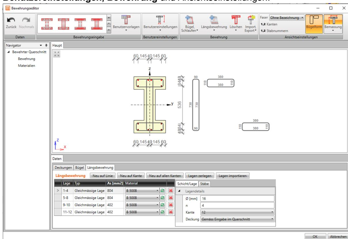
The screenshot displays the 'Bewehrungseditor' software interface. The main window shows a cross-section of a reinforced concrete beam with dimensions and reinforcement details. The 'Daten' (Data) tab is active, showing a table for longitudinal reinforcement (Längsbewehrung) and a 'Lagendetails' (Reinforcement Details) panel.
