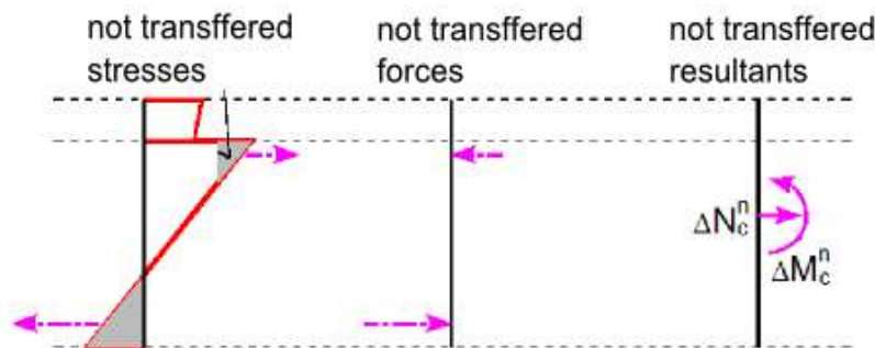
Fig. 1.11 – Not-transferred inner forces [4]
