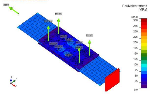
Check of preloaded bolts for extreme load effect
