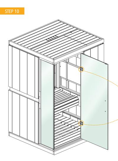
Using the Allen wrench 6, you will tighten the bolts into the hinges as the door L is inserted. Make sure the bolt is inserted firmly. Each hinge will have four plastic gaskets. The door will be inserted between the four gaskets.
